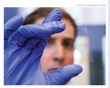
Graduate student Nicholas Davy holds a sample of glass that uses near-ultraviolet light to generate electricity, which powers chemical reactions that lighten or darken the glass.
